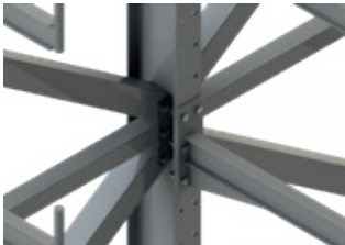
YATAY VE DİYAGONAL ÇAPRAZ KONNEKTÖRLERİNİN MONTAJI / MOUNTING OF HORIZONTAL AND DIAGONAL CROSS-CONNECTORS
